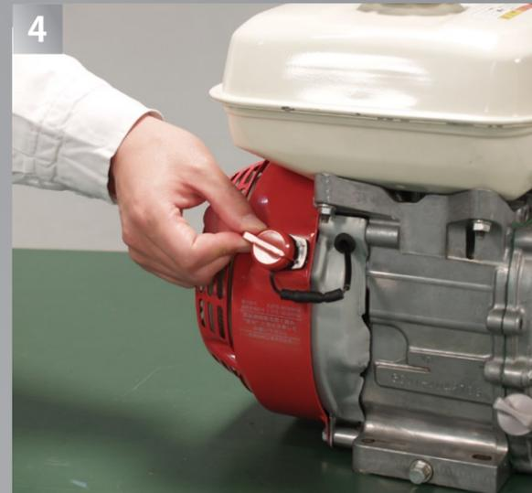
Turn the engine switch to the ON position.
