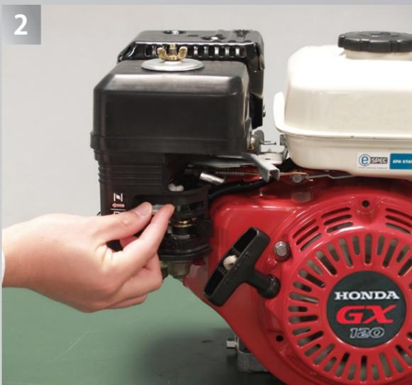
Move the choke lever to the CLOSED position.
