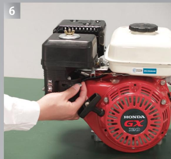
Gradually move the choke lever to the OPEN position as the engine warms up.
