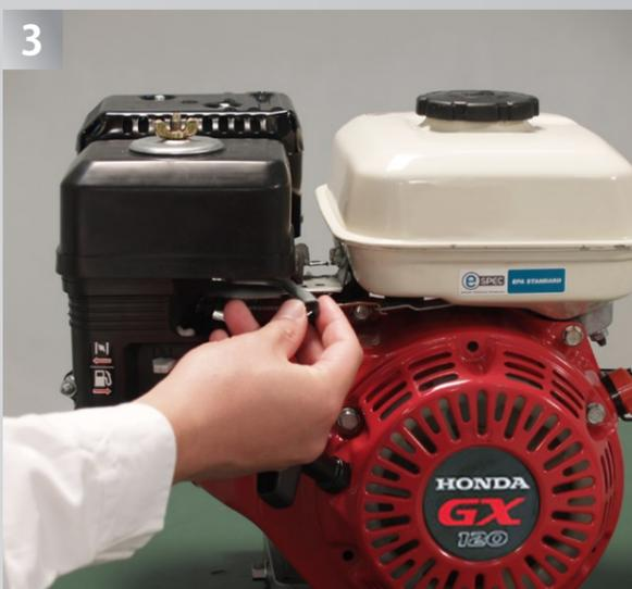
Move the throttle control lever slightly to the left.
